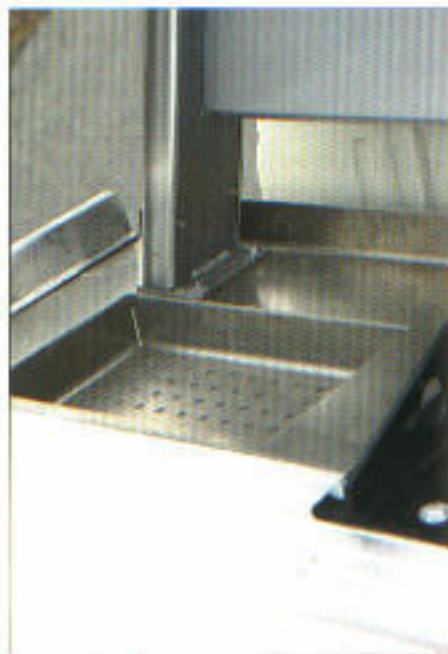
Large chain trays with drain holes
